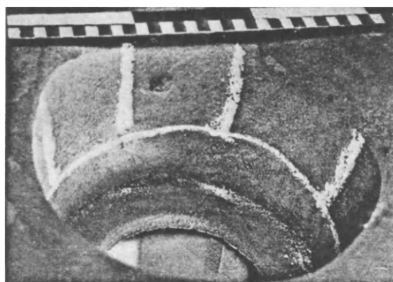
FIG. 403. Remedy—easily visible marks on the feeder head.
