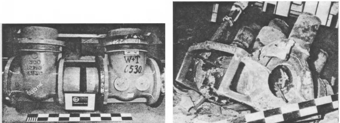
FIG. 428. Pattern (top) and undressed casting (bottom) of a gate valve casing, using exothermic pads.
