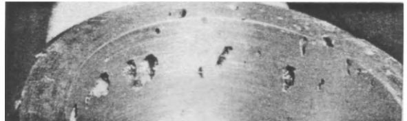
FIG. 450. This lever arm (made without exothermic pads) also exhibits a typical enrichment of pores near the feeder head.
