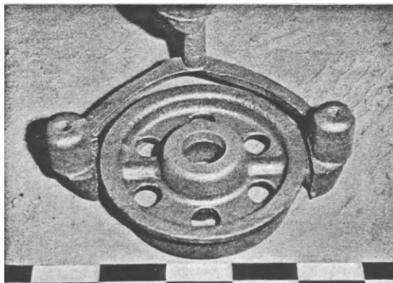
FIG. 197. Method of moulding wheels with feeding webs, Washburn cores and blind feeder heads.
