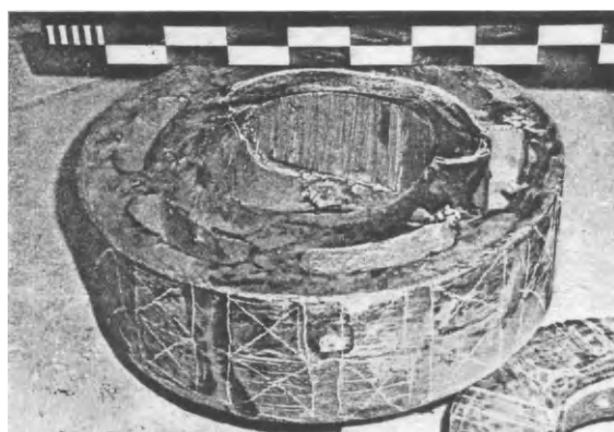
FIG. 289. Massive toggle, heavily chilled on economic grounds. Note the small feeder head.
