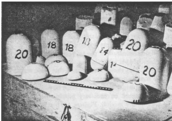
FIGS. 101 b and c. Various standard feeders (see Tables 9-19) for selecting from the point of view of moulding technology.
