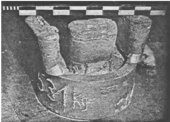
FIGS. 159b and c. Brake drums. b. With two rim and one boss feeder. c. Rim and boss fed by a single side feeder. An artificial end zone produced at the rim (see Chapter 8).
