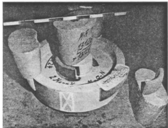
FIG. 443a. Use of exothermic pads on the boss of a gear wheel. The use of exothermic feeder heads is not necessary for this purpose, as the above example shows.
