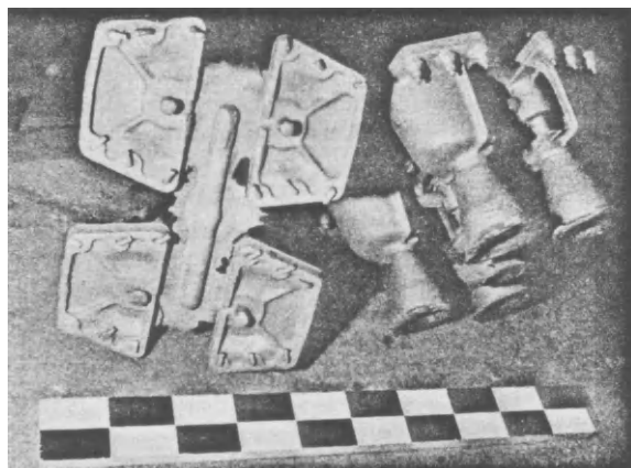
FIG. 314d. Internal chills in the lugs of LKW. The chills stand vertically in the casting.
