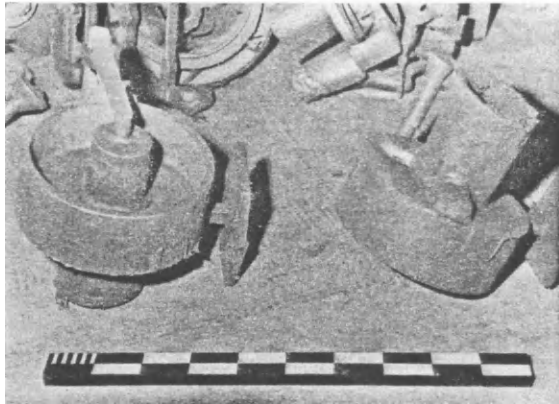
FIG. 159a. The rim section of a brake drum was fed through shoulders from the boss feeder head.
