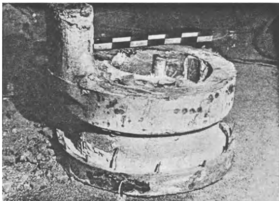
FIG. 246 a. Boss with internal gear, fed with only one feeder head and extended artificial end zones.
