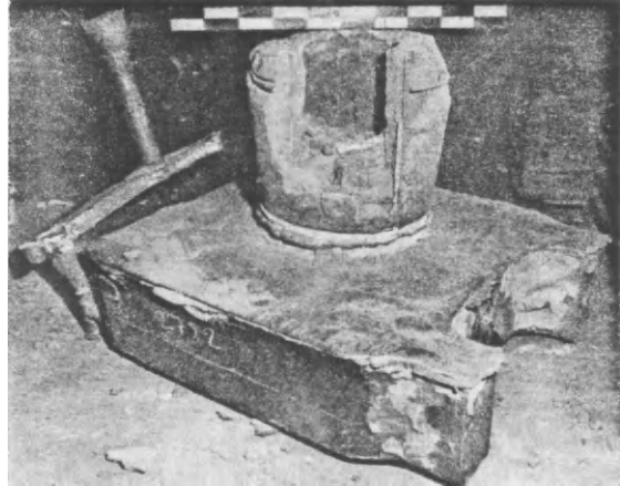
FIG. 344 a. Horizontal sinking of the metal surface of an exothermic feeder head on a large squeezer plate (for a press).
