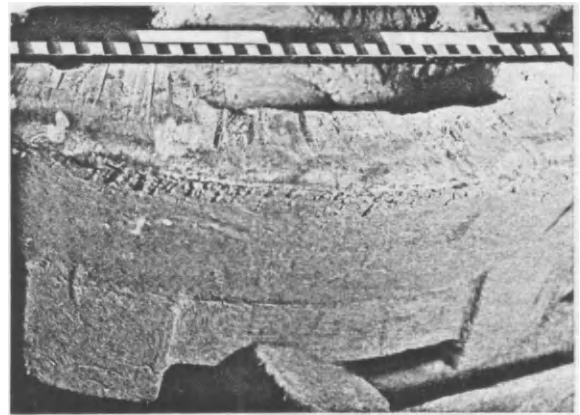
FIG. 368b. Tup for a scrap plant. Fed by means of an exothermic feeder head. No internal chills were inserted in the casting.
