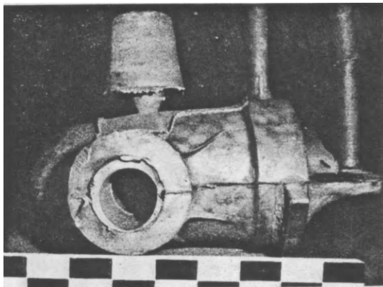
(c) and (d) Detail photographs of the feeder head neck and the exothermic pad surface.
