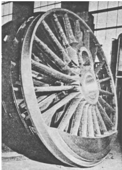
FIGS. 239a and b. Locomotive wheel centre. (a) without and (b) and (c) with artificial end zones. With this order alone the method used in (b) and (c) gave a saving of £ 2500 in melting costs.
