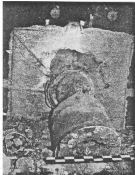
FIG. 344 a. Horizontal sinking of the metal surface of an exothermic feeder head on a large squeezer plate (for a press).
