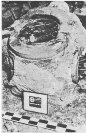
FIGS. 429a-b. (a) Pattern of a pipe fitting with an exothermic pad inserted as a core. (b) Undressed casting. The finished casting was ultrasonically sound.
