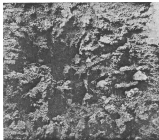
FIG. 39. Dendrites from a shrinkage cavity. (a) from a “cupola scaffold”; (b) from a horizontal “runout” (see also Fig. 72).
