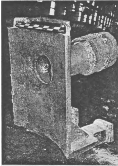
FIGS. 406a and b. Trunnion plate of a casting ladle. a. without and b. with exothermic feeder heads.
