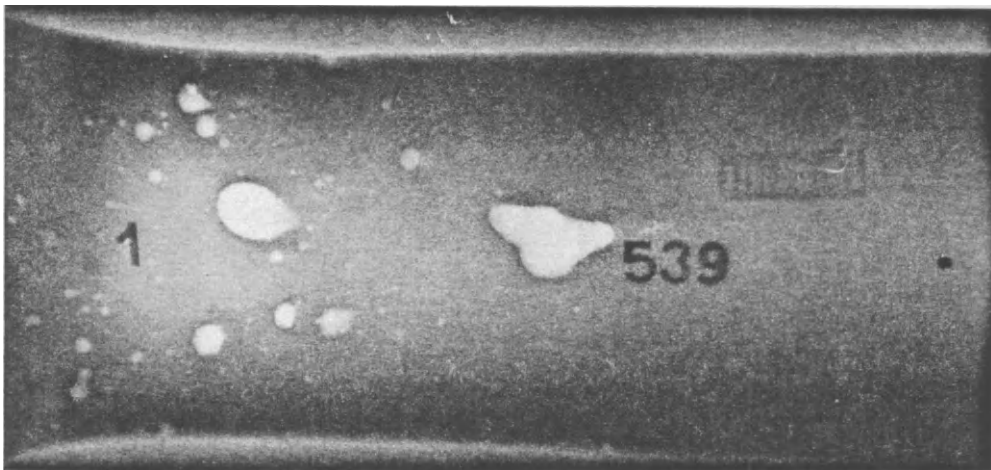
FIG. 465. X-ray photograph of typical slag blowholes in a gear wheel rim.
