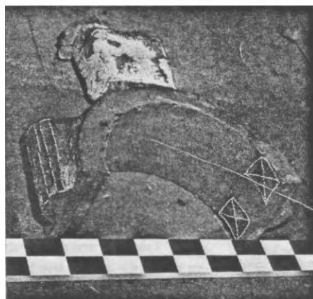
FIG. 113b. The massive eye lugs are cooled with chills. (This casting is not identical with that shown in Fig. 126b.) (Courtesy SULZER Bros.)
