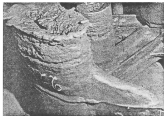
FIG. 149. Correct runout of the shoulder.
