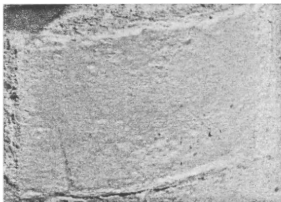
FIGS. 259a and b. A test was carried out by placing a shot blasted and a scaled chill on the same casting. The gases at the scaled chill led to the formation of wormholes on the surface of the casting. The pores were up to 40 mm deep
