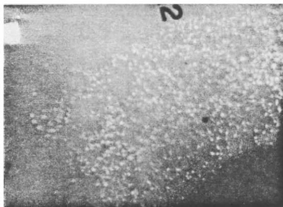
FIG. 265 a. Sharply delineated zone of porosity under a ring chill. Porosity was also found on the same casting at thin sections with a high rate of solidification.
