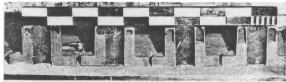
FIG. 82b. Cavities in flanges, bounded by a horizontal base, produced by incomplete filling, and erroneously termed "blow-holes".
