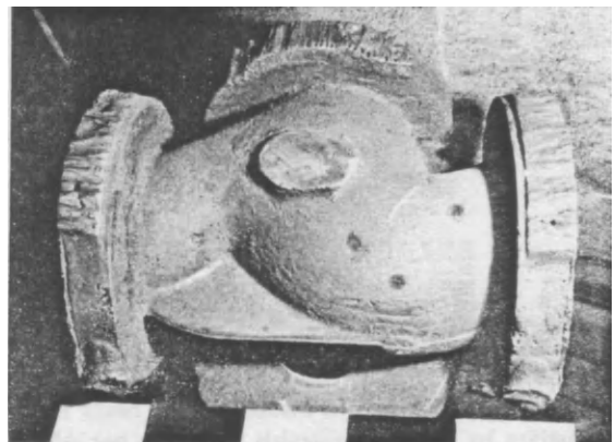
FIG. 447. Porosity at the surfaces of application of exothermic pads. The charge of metal represents a boundary case of the so-called "cauliflowing". Note, however, the concentration of pores on the sand side of the central flange.
