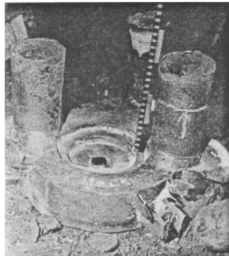
FIG. 83. Waste of steel due to overfilling the feeder.
