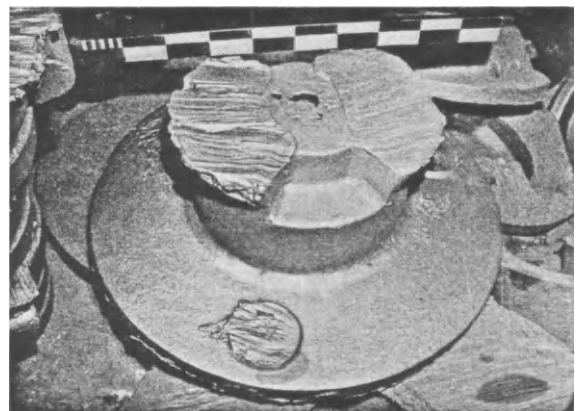
FIG. 51. Waste of steel caused by using two feeders inside a single feeding area on the boss of a flange coupling. The flange feeder was incorrectly dimensioned, resulting in cavities (cf. Fig. 237).
