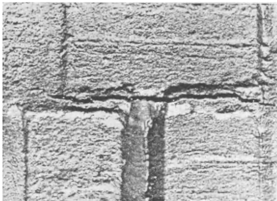
FIG. 275. Formation of burrs on chills as a result of slipshod ramming, with consequent hot tearing.
