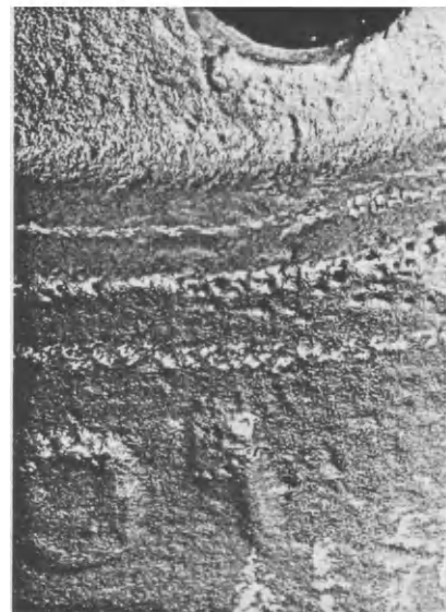
FIGS. 264 a and b. When the steel melting practice is unsatisfactory, porosity occurs preferentially at all positions with a higher solidification rate, such as fins, fillets, pattern numbers, etc.
