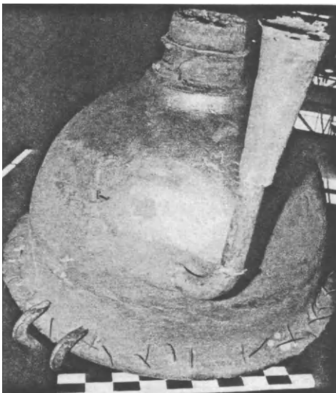
FIGS. 372a and b. Guide pulley (a) without, (b) with exothermic feeder heads and intermediate chills. Note the considerable withdrawal of metal from the exothermic feeder heads.
