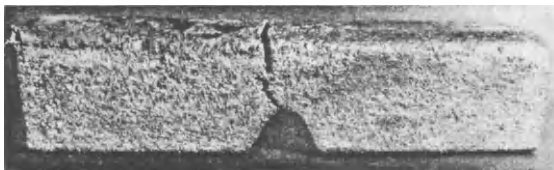
FIG. 268. Test piece for the rapid determination of the gas content of steel.
