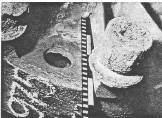
FIGS. 369a-d. Crane pulley, a and b without, c and d with, exothermic feeder heads. By using these feeder heads working time was also saved in the dressing shop, and less machining was required.
